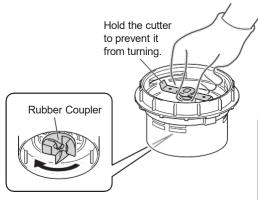
Fix the cutter shaft on the back side of the cup holder with a flat-blade screwdriver, etc., and turn the cutter in the direction of the arrow in the figure to remove it
