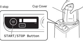
Unplug the power plug from the outlet after the cutter has completely stopped rotating. Remove the cup cover in the reverse order of attaching, and remove the cup and the cup holder from the main unit.
